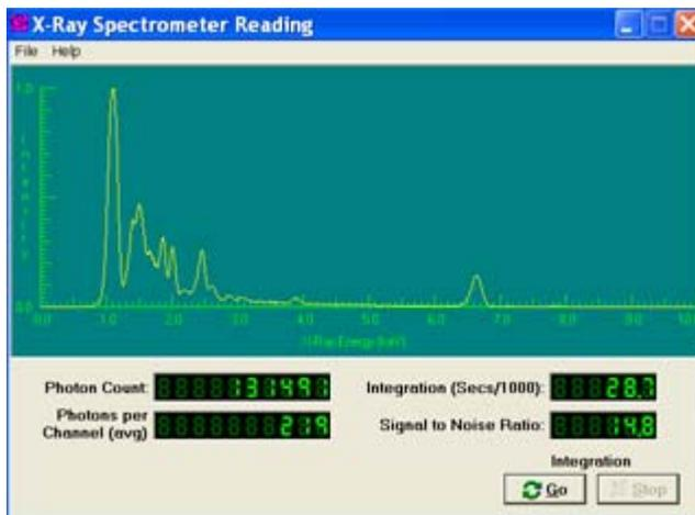
To take a spectrum, simply click on the **Go** button. The spectrum can be seen building up, photon by photon, as the exposure increases. To stop the exposure, simply click the **Stop** button. Exposures can be continued by simply clicking **Go** again.
